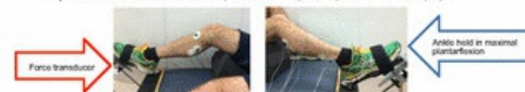
Figure 3. Experimental set up. Six recording EMG electrodes were affixed to all three heads of the triceps surae. EMG and muscle force were continuously measured during MVC and throughout the muscle cramp.
